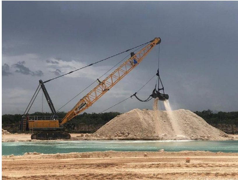
Picture 5 - Dragline Extracting Below-Water Shot Rock
