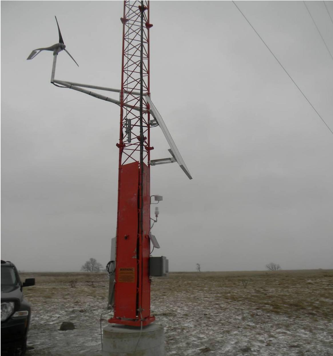
**Figure A.10 - Solar Panels, Wind Turbine, Battery Bank, Logger Enclosure, Satellite Antenna and Temperature Sensor at the Mast Base**
