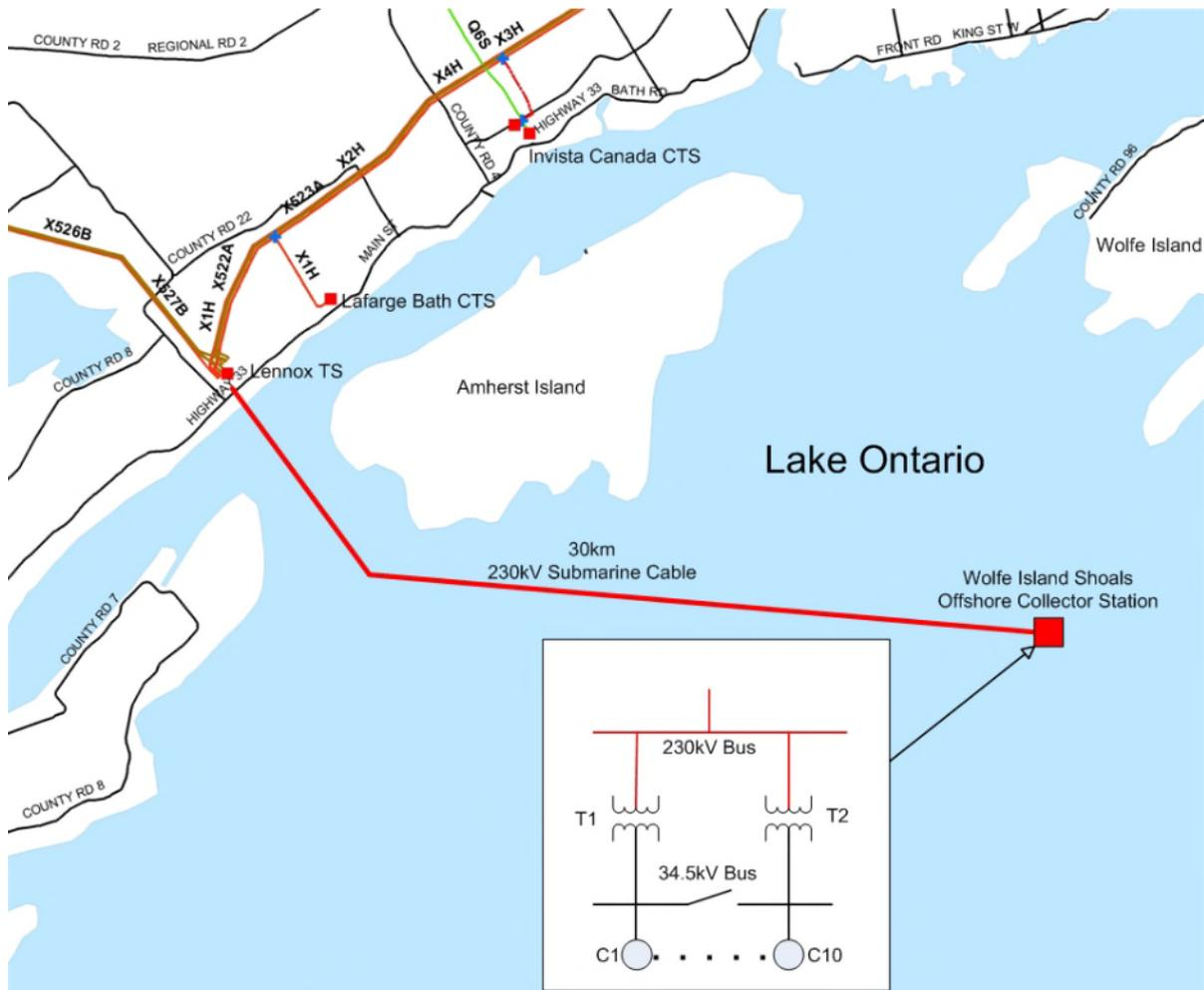
**Figure A.51 - Approved Connection between Wolfe Island Shoals (offshore) substation and Lennox (onshore) Generating Station**
