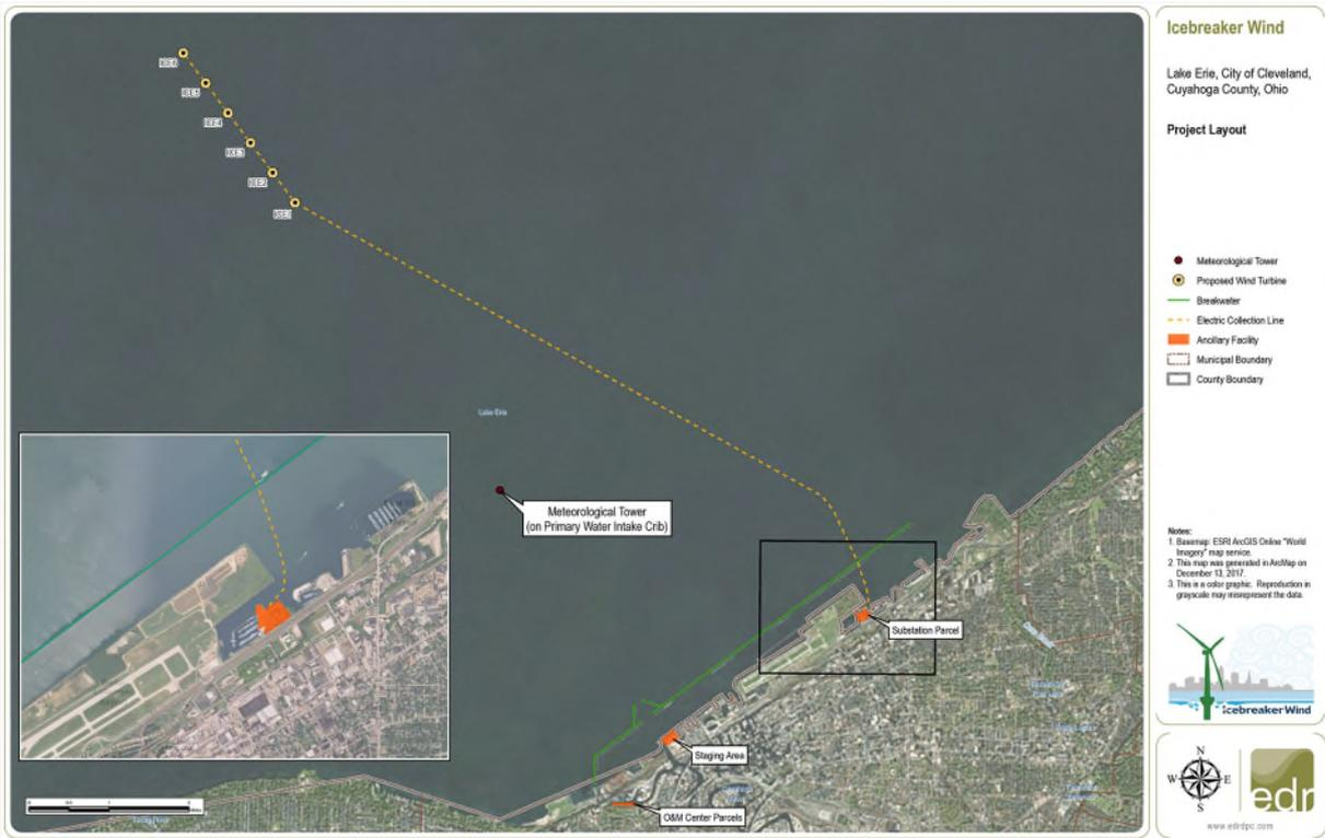
**Figure A.63 - Approved LEEDCo Icebreaker offshore wind project plan, Lake Erie**
