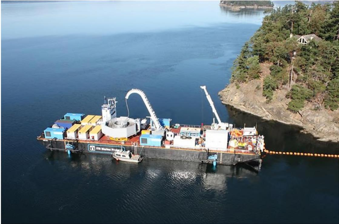
**Figure A.59 - Cable Installation Barge Shore Landing**
