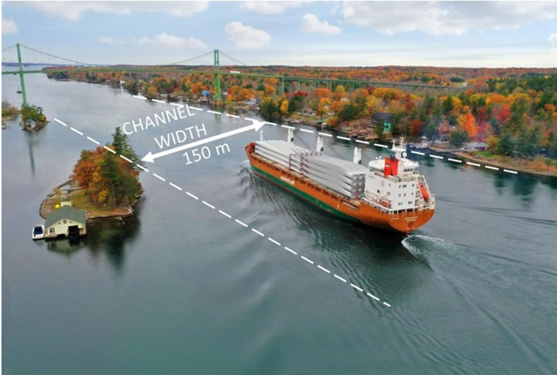
**Figure A.75 - Vessel Carrying Wind Turbine Blades Passing Through Existing American Narrows Channel for Two-way Traffic**
